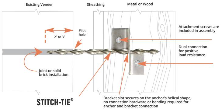
Install anchor first within 1" from stud THEN install the bracket
